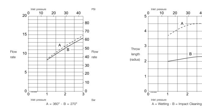
For Clip-on models, the flow rate is increased by approx. 1.5  $m^3/h$ .
