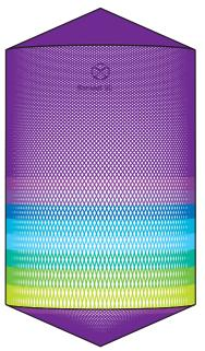
D2m H3m, Toftejorg SaniJet 20, 4 x  $\emptyset$ 4.2 mm, Time = 7.6 min., Water consumption = 763 l
