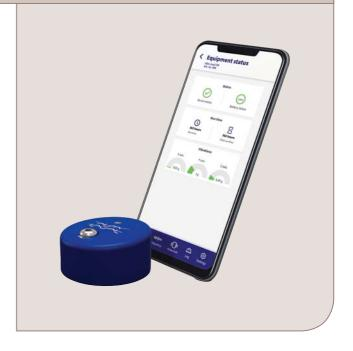
When the monitor senses some vibration it activates, starts the running hours counter and monitors the tri-axial vibration and internal temperature of the unit at pre-set intervals determined by the user. This information is sent via Bluetooth to a mobile device running the application if within 20 meters of the condition monitor.
