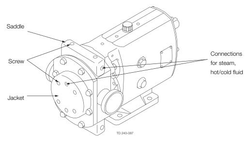
The maximum allowable pressure and temperature of heating/cooling fluid is 3.5 bar and  $150^{\circ}$ C respectively, except in T4 applications in which the maximum allowable temperature is  $115^{\circ}$ C.
