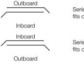
Series 1, the outboard seal fits over the inboard seal.
