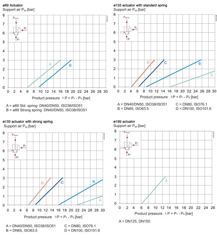
Upper plug max. product pressure against which the valve can open, as a function of air pressure:
