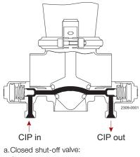
Cleaning of the leakage chamber.
