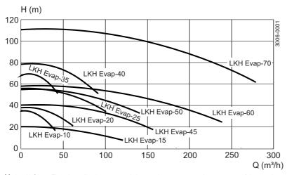
Note: If Clear Flow impeller is mounted the performance can be up to 10% lower than shown on the curves above
