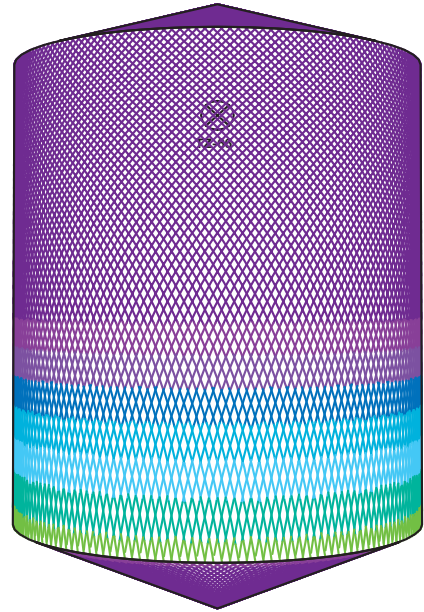
D8m H10m, Toftejorg TZ-66, 4 x \varnothing 10 mm, 0% Time = 23.3 min., Water consumption = 10868 l
