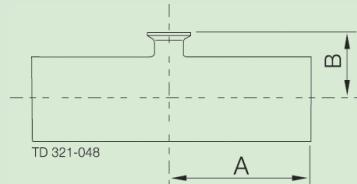
**RACCORD EN T SOUDURE COURT/CLAMP/SOUDURE TRI-CLOVER CDE B7RWWMS ASME BPE
