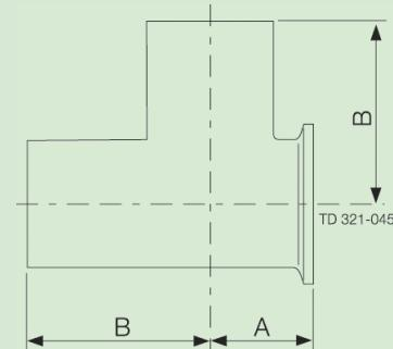
**RACCORD EN T SOUDURE/CLAMP/SOUDURE "OUTLET RUN" TEE TRI-CLOVER CODE B7WMSW ASME BPE
