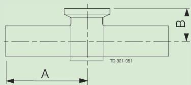
**RACCORD EN T POUR INSTRUMENTS LLC WWC TRI-CLOVER CODE B7IWWMS ASME BPE CODE DT-4.1.2-10**
