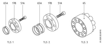
• TLS 1 y TLS 2: the adjustable fastening system is made up of three parts: Allen screws (51A), conical tightening rings (65A) and dragging bushing (17B).
