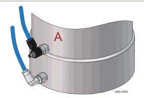
2 Adjust to the desired valve speed by turning the adjustment screw on the throttle valve.
