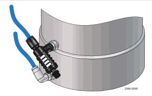
2 Adjust exhaust air flow with the adjustment screw. Then use the locking nut to secure the position of the adjustment screw.
