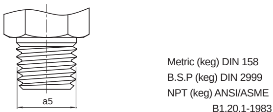
Form C (DIN 3852 Part 1&2) with sealing in tapered thread
