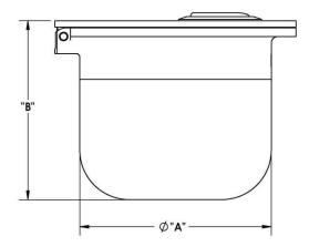
Material: 316L Stainless Steel Roughness: ≤ 20 Ra (Internal)
