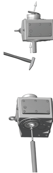
Figure 3-5: Removing the factory-fitted closing cap
