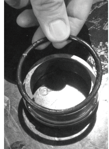
Figure 10, O-ring for seal part 30B
