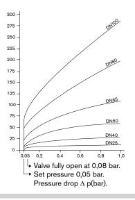
This diagram shows the flow characteristics depending on the pressure drop
