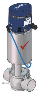
2 Verify that the air exhaust plug points downwards as indicated by the arrow to avoid water ingress in the pneumatic system. You can rotate the exhaust plug until it points in the right direction.
