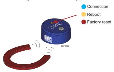
In case the CM becomes unconnectable via the Alfa Laval Condition Monitor application the CM firmware can be restarted by holding a magnet to the QR code located on the CM.
