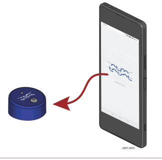
Wake up the CM by shaking it, until the LED flashes blue or hold a magnet to the QR-code until the LED flashes blue, then remove the magnet.
