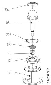
See section 9.7. Exploded drawing and parts list of the INNOVA G valve for a reference to the parts described.
