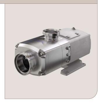
The front-loading, self-setting cartridge design makes it easy to replace the shaft seal while the pump is in place. Single, single flush and double mechanical cartridge seals are available. All options are fully front-loading and interchangeable.
