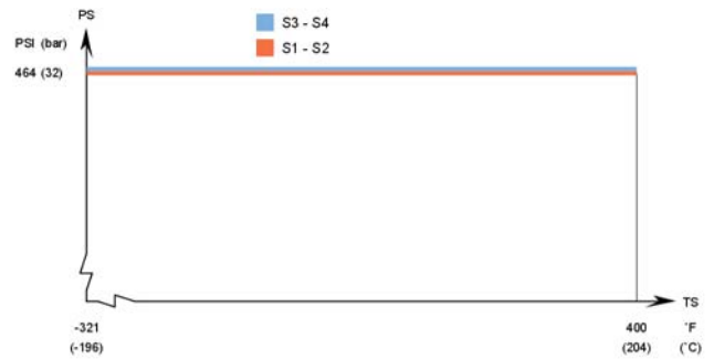
CB112AQ – UL approval pressure/temperature graph
