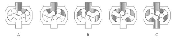
**A**: When the lobes rotate, the space on the suction side increases because one lobe moves away from the other, thus causing a partial vacuum that draws the liquid into the pumping chamber.
