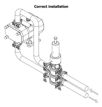
Example of standard Pressure Relief Valve installation. This arrangement creates a dead leg with a large amount of product. Example of Hygienic NCS Pressure Relief Valve installation, with air actuated rising.
