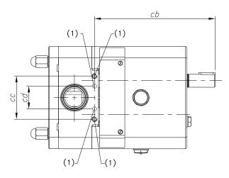
(1) Flushing sealing connection 4 x G1/8"
