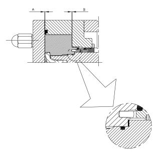
This is the final adjustment to be carried out. The pump must be synchronised and the pump rotor case must be mounted on the gear case.
