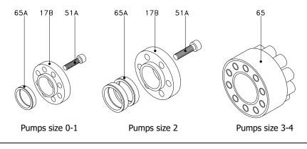
**Pumps Size 0, 1, and 2:** the adjustable fixing mechanism consists of three pieces: Allen screws (51A), bearing cones (65A), and impeller bushing (17B).
