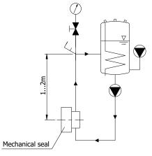
Pressure tank connection lay out
