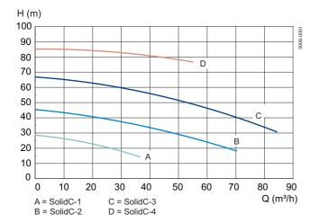
Frequency: 60 Hz Speed (synchr): 3600 rpm
