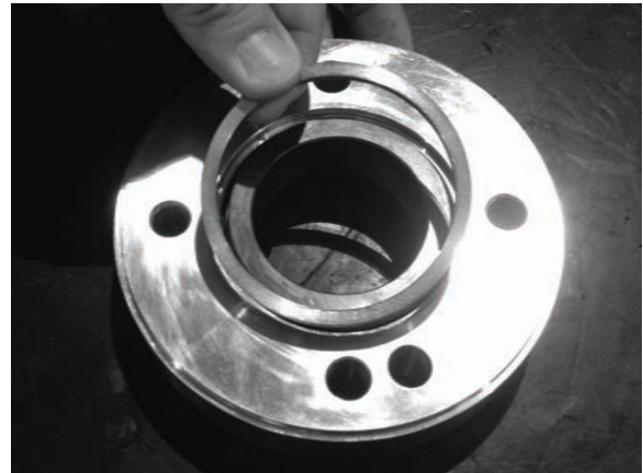
Figure 12, Gasket support in place
