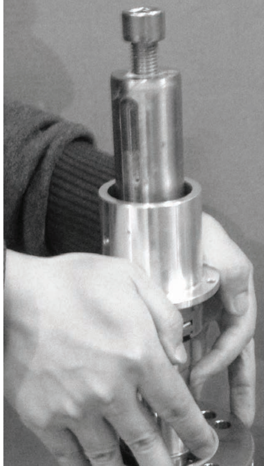
Figure 10, Pressing down the seal
