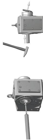
Figure 3-5: Removing the factory-fitted closing cap
